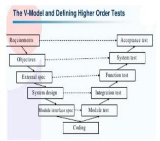
Fig. 4: For V-Model Testing.
