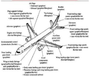
Fig. 1: For Exterior Parts of the Aircraft.
