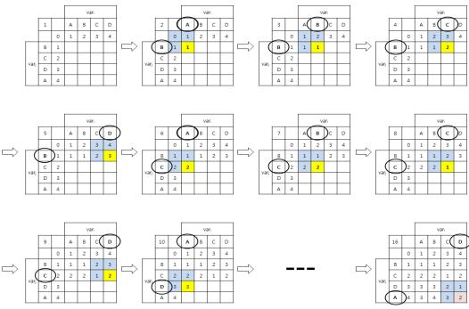
Fig. 1: Process of Measuring Levenshtein Distance [7].
