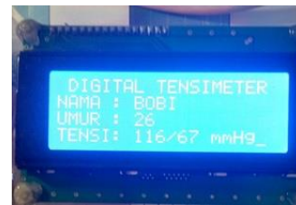
Fig.5:16x4 LCD Testing
