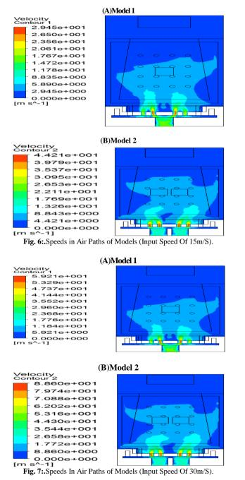
Fig. 6 and Fig. 7 show the speeds for both of the models. Fig. 6 shows the speeds at the wind speed of 15m/s for the inlet, marking the maximum speed of 29.45m/s for model 1. Model 2 also marked a speed of 44.21m/s. Fig. 7 shows the speeds at the wind speed of 30m/s at the inlet. It shows that model 1 showed a speed of 44.21m/s and model 2 marked the speed of 88.60m/s,
