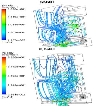
Fig. 5:.Speeds in the Entire Shapes of Models (Input Speed of 30m/s).
