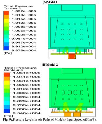
Fig. 8 and Fig. 9 show the pressure levels in air patch at different wind speeds, and Fig. 8 applied a speed of 15m/s to the air inlet. Here, model 1 showed the maximum pressure of 100.60kPa. Model [2] also got a pressure of 101.30kPa. Fig. 9 shows the resulting values with the inlet set at 30m/s, and model 1 showed a pressure of 102.20kPa while model 2 showed a pressure of 105.10kPa. We saw that both resulting values showed the greatest pressure at the junction of air blower and air path.
