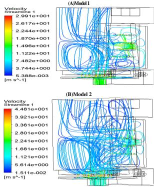
Fig. 4:.Speeds in the Entire Shapes of Models (Input Speed of 15m/s).
