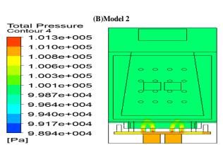
Fig.: 8. Pressure Levels in Air Paths of Models (Input Speed of 15m/S).
