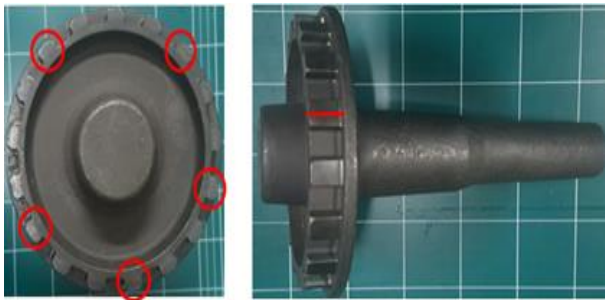
Fig. 21: Surface Roughness Measurement of the Final Prototype
