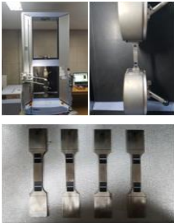
Fig. 4: Tension Testing Machine and Samples.
