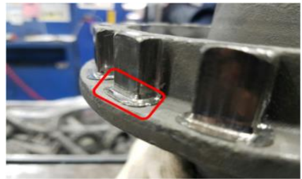
Fig. 17: Defects in Cold Forging.
