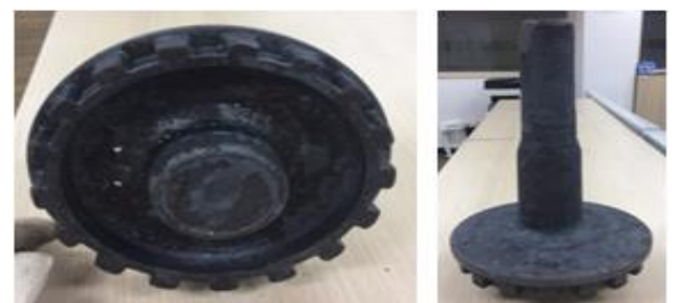
Fig. 14: Hot Forging Press Mold and Prototype.
