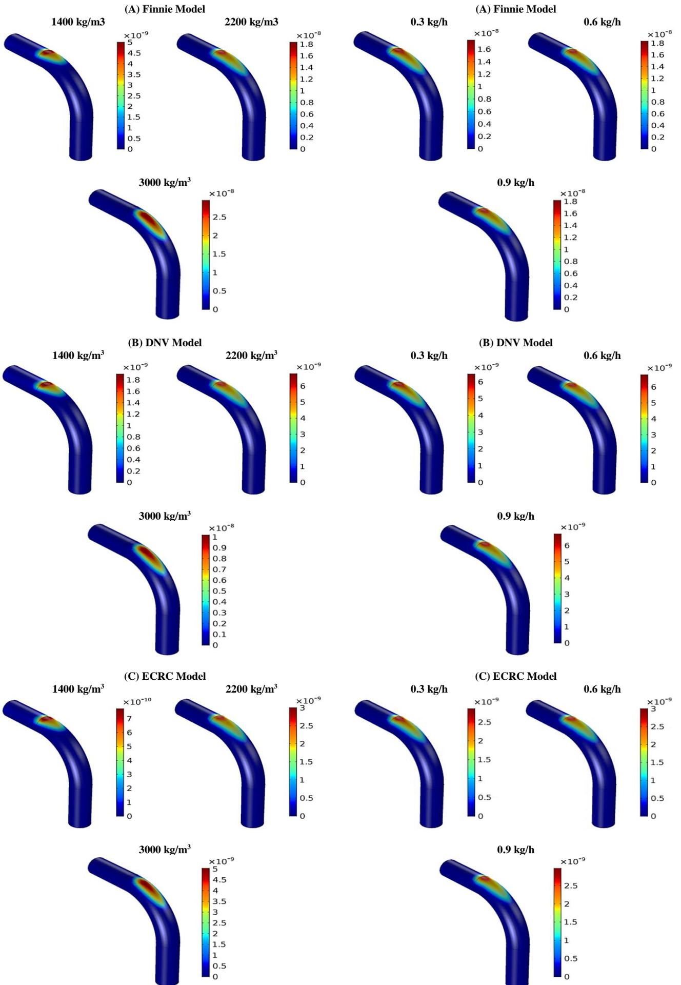
Fig. 8: Erosive Wear Rate [Kg/m<sup>2</sup>.s] for Different Sand Particles Density.
