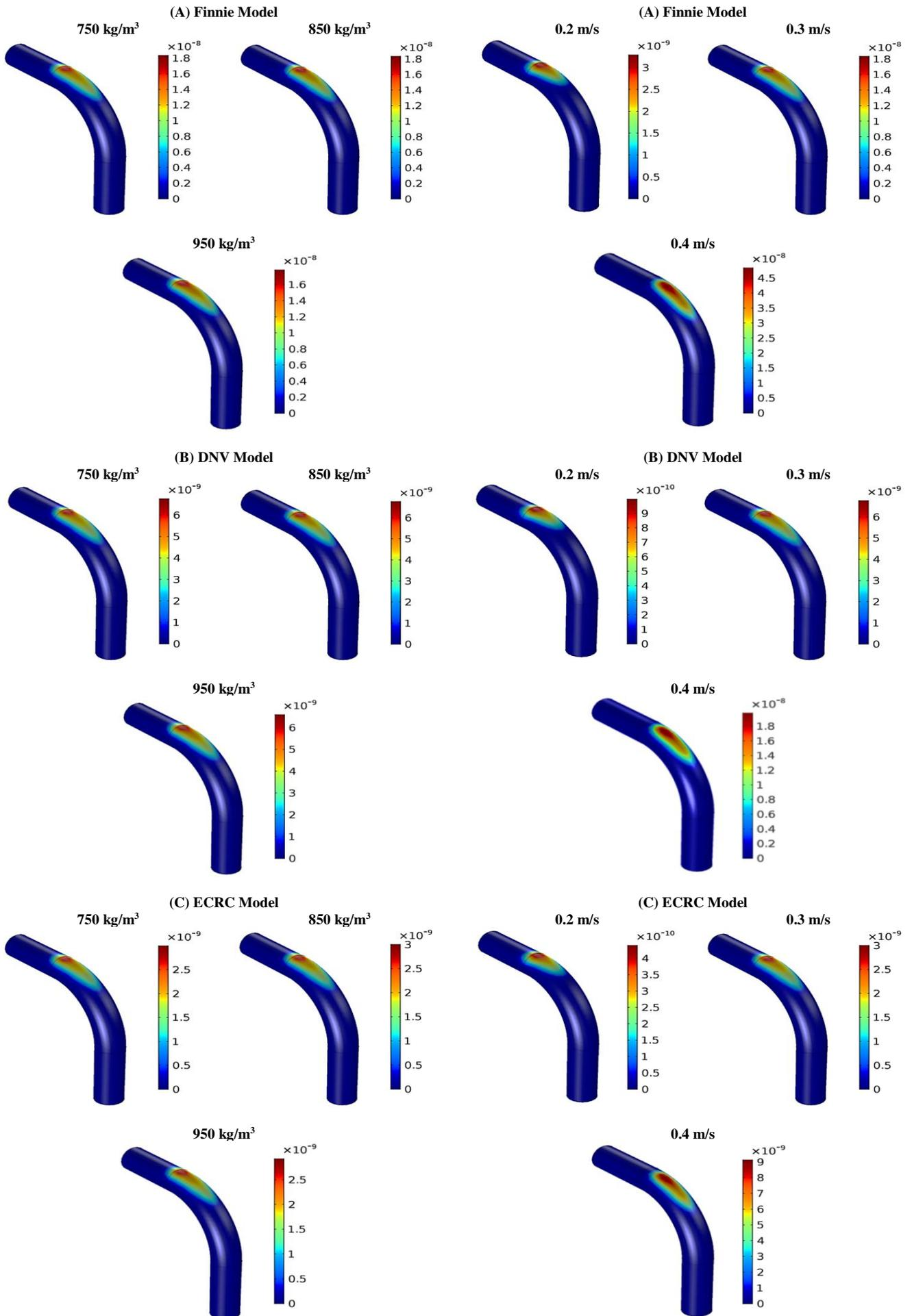
Fig. 4: Erosive Wear Rate [Kg/m<sup>2</sup>.s] for Different Values Fluid Density.
