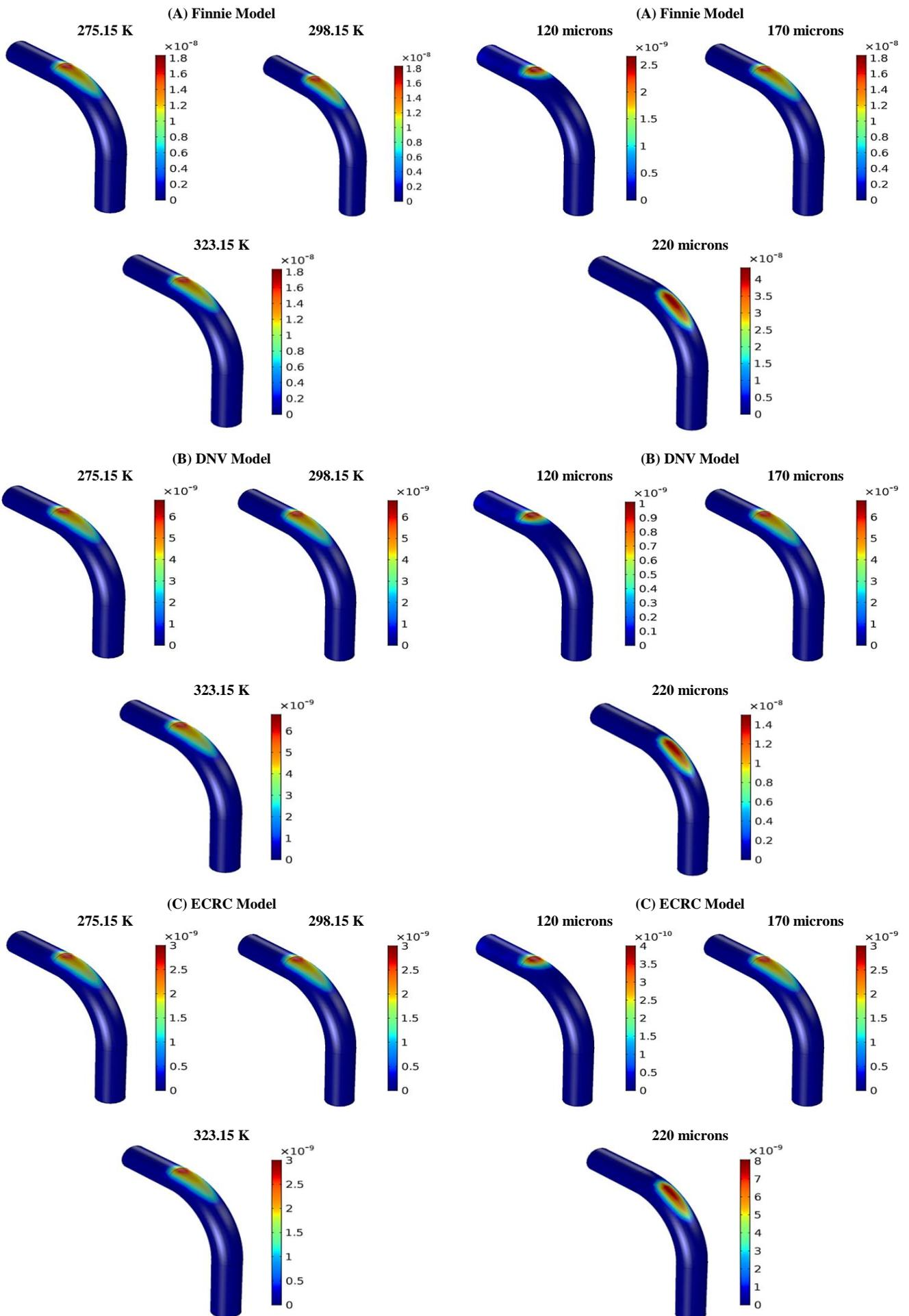
Fig. 6: Erosive Wear Rate [Kg/m<sup>2</sup>.s] for Different Fluid Temperature.
