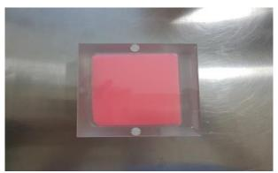
Fig. 3: Breast Equivalent Material Phantom.
