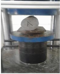
Fig. 2: Splitting tensile test set-up
