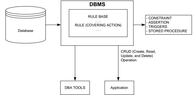
**Fig. 2:** Active Database Architecture
