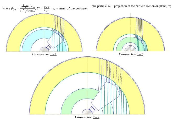
Fig. 2 The motion path of the concrete mix particles when descending from the screw blades of the drum and spiral-blade shaft of the concrete mixer truck not tacking into account the environmental resistance in three different section of the drum
