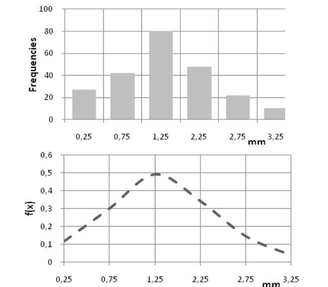
Fig. 4: Histogram and graph of distribution density of geometric deviations of brick length
