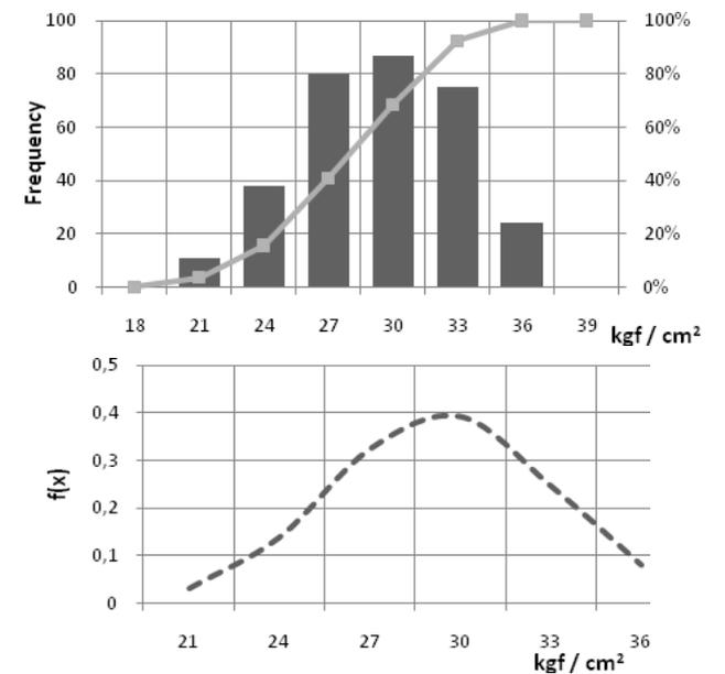
Fig. 3: Histogram and graph of distribution density of the strength of bricks for bending
