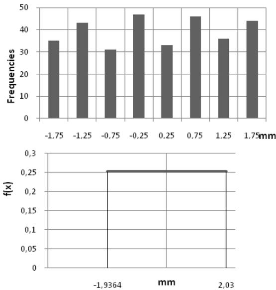
Fig. 5: Histogram and graph of distribution density of geometric deviations of brick height
