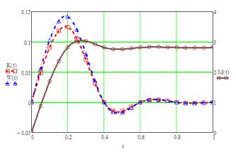
**Fig.4:** Changing the angular accelerations of the rotor electric motor  $K(t) = \phi_1^{\text{"}} = D^{\text{'}}(t) = Z^{\text{"}}(t)$ ,  $\operatorname{rad/s^2}$ , the unbalanced shaft  $W(t) = \phi_2^{\text{"}} = N^{\text{'}}(t) = Q^{\text{"}}(t)$ ,  $\operatorname{rad/s^2}$ , and the moment of the vibrator drive motor M(t),  $N \cdot m$ , depending on the time t, s (without a declining)
