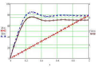
**Fig. 2:** Change of angular mass transfer  $Z(t) = \phi_1$ , rad, angular velocity  $D(t) = Z'(t) = \phi_1'$ , rad/c, and the moment of the motor drive vibrator M(t), N·m, depending on time t, s (without declining)
