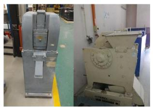
Fig. 2: Jaw Crushers at the UITM Laboratory Treatment of CCWA.
