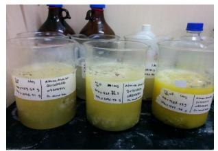
Fig. 3: Specimens of CCWA Soaked the HCL with Different Molarity.
