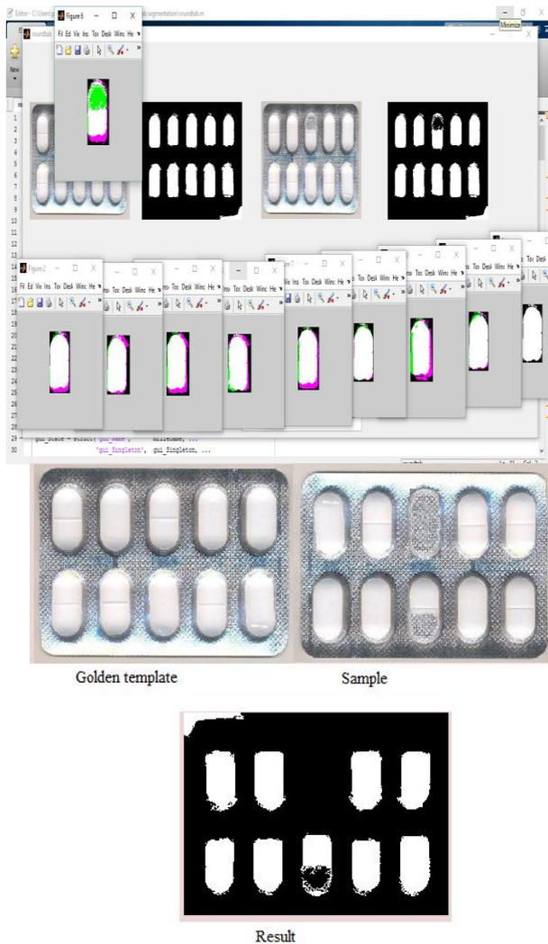
Fig.4: Segmentation and comparison for oval shaped tablets detection.
