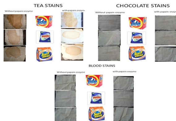
Fig. 12: Removal of tea, chocolate and blood stains using papain like enzyme from betel leaves Pieces of populine cloth were overnight stained with tea, chocolate and blood stains. They were washed with three different detergents TIDE, HENKO, SURF EXCEL. Three controls were set without papain like protease. For the test samples Papain like protease was added. Test samples showed effective destaining when compared with controls.
