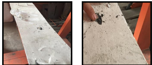
Fig. 9: Penetration Hole at the Top Face of the Specimens.
