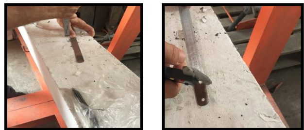
Fig. 10: Manual Methodology to Measure the Depth and the Diameter of the Penetration Hole.
