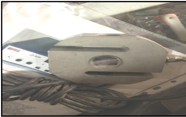
Fig. 5: Load Cell Record the Applied Load.
