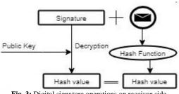
Fig. 3: Digital signature operations on receiver side
