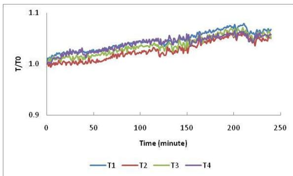
Fig. 5: Temperature profile for panel without composite
