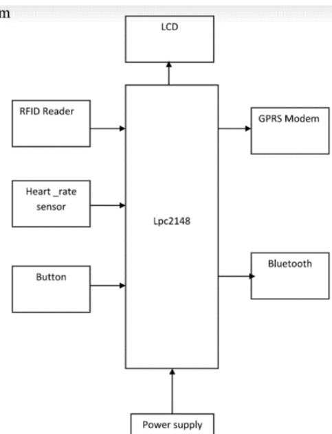
Fig. 2: Device to Authenticate.
