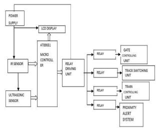
Fig. 3: Diagram of Automated Railway System.
