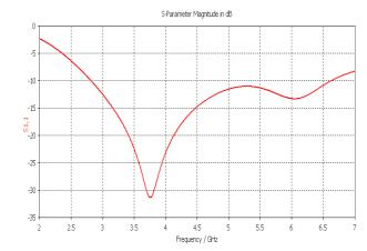
Fig. 2: Return Loss vs Frequency Plot of Proposed Antenna.
