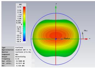
Fig. 6: Far Field 3-Dimensional Radiation Pattern Showing Directivity of Proposed Receiver Antenna.
