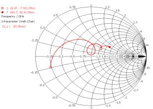
Fig. 4: Smith Chart vs Frequency Plot of Presented Receiver Antenna
