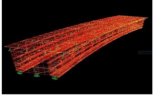
**Fig. 2**: Steel – composite tub girder modelled in SAP2000
