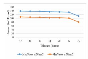
Fig. 10: Stress V/s thickness of bottom stiffener, when vehicle loading is given to only one girder
