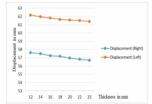
Fig. 8: Displacement V/s thickness of vertical stiffener, when vehicle loading is given to only one girder
