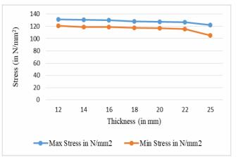
Fig. 12: Stress V/s thickness of web stiffener, when vehicle loading is given to only one girder  $\$
