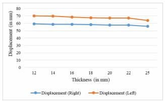
Fig. 5: Displacement V/s thickness of web stiffener, when vehicle loading is given to both girders
