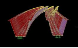
Fig. 1: Steel girder with stiffeners modelled in SAP2000
