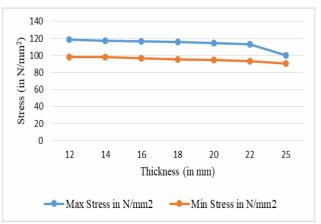
Fig. 14: Stress V/s thickness of vertical stiffener, when vehicle loading is given to only one girder
