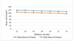
Fig. 9: Stress V/s thickness of bottom stiffener, when vehicle loading is given at both girder
