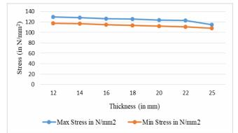
Fig. 11: Stress V/s thickness of web stiffener, when vehicle loading is given at both girder
