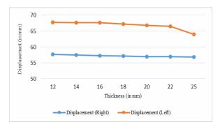
**Fig. 7:** Displacement V/s thickness of vertical stiffener, when vehicle loading is given to both girders
