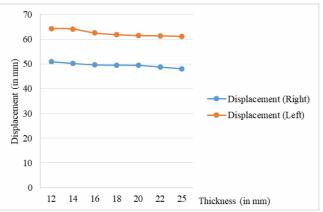
Fig. 6: Displacement V/s thickness of web stiffener, when vehicle loading is given to only one girder
