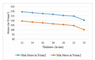
Fig. 13: Stress V/s thickness of vertical stiffener, when vehicle loading is given at both girder
