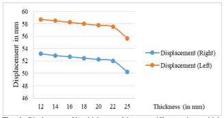
Fig. 4: Displacement V/s thickness of bottom stiffener, when vehicle loading is given to only one girder
