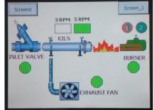
Fig. 5: Front pannel HMI screen
