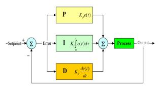
Fig. 4: PID Controller action
