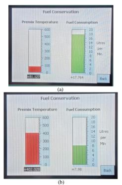
Fig. 6: Fuel Consumption based on recovered heat (a) At Minimum Temperature, (b) At Maximum Temperature
