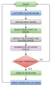
Fig. 2: Flowchart of the algorithm
