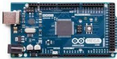
Figure 2.4: Arduino mega
