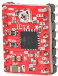
Figure 2.3: Stepper motor module
