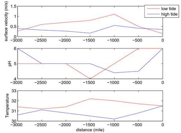
Fig. 2: The water mass (velocity, pH and temperature) observation in Kampar River during low tide and high tide at June, 16-17 2016. The distance measure from the last station (no.7) to the first station (no.1) upstream ward.
