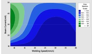
Figure 4: Contour plot of grey relation grade Vs beam current and welding speed
