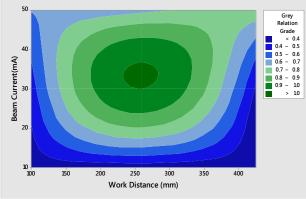
Figure 5: Contour plot of grey relation grade Vs beam current and work distance
