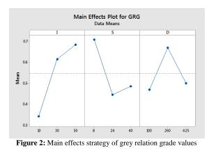
From the above plot it was found that the optimum input values of beam current, welding speed and Working distance are 50 mA, 8 mm/s and 260 mm.
