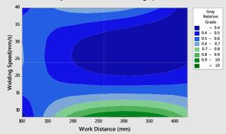
Figure 6: Contour plot of grey relation grade Vs welding speed and work distance
