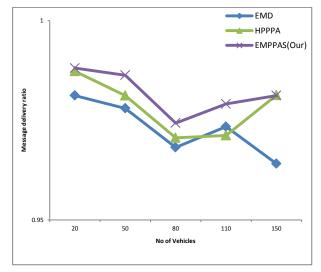
Fig. 5(b): Comparison of message delivery ratio among different schemes
