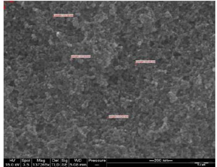
Figure 2 SEM morphology of Magnetite nanoparticles
