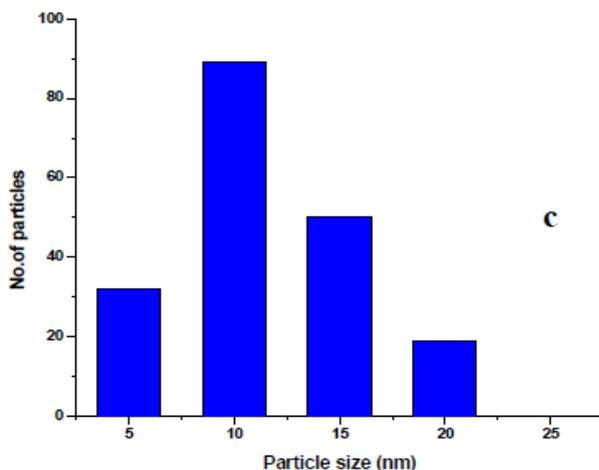
Figure 1 (a) & (b) Non-contact mode AFM image of scan size 3  $\mu$ m, showing spherical magnetite nanoparticles and (c) Histogram of magnetite particle size distribution
