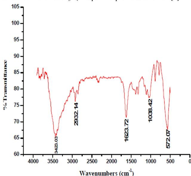
Figure 5 FTIR Spectrum of magnetite nanoparticles
