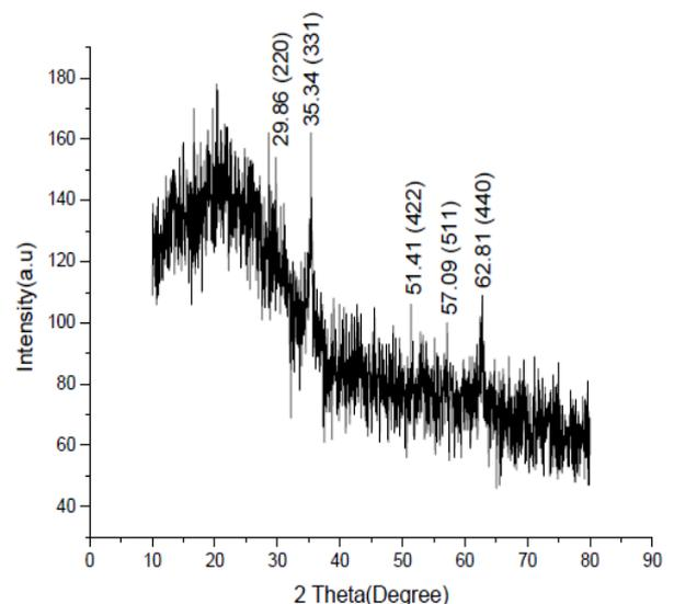
Fig 3 X-Ray diffraction patterns of the Fe<sub>3</sub>O<sub>4</sub> nanoparticles
