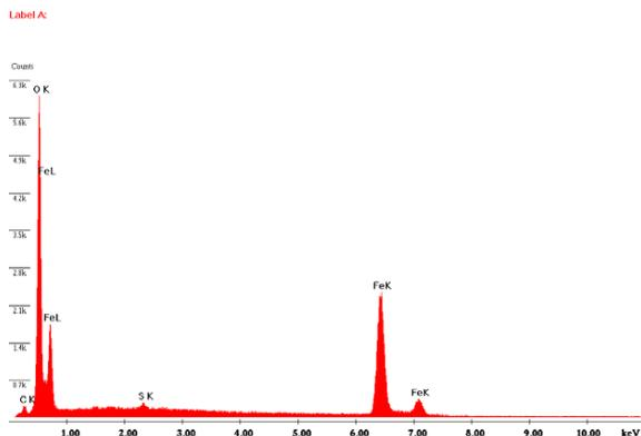
Figure 4 The EDAX Spectrum of synthesized  $\text{Fe}_3\text{O}_4$  nanoparticles
