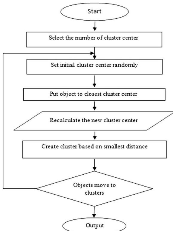
Fig 1 Flowchart of k-means clustering algorithm
