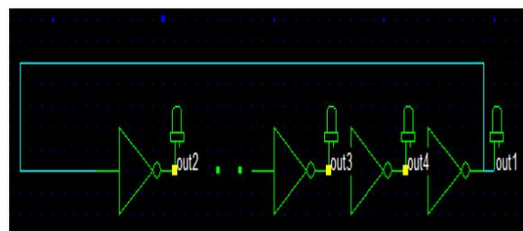
Fig. 1: Inverter chain to form ring oscillator
