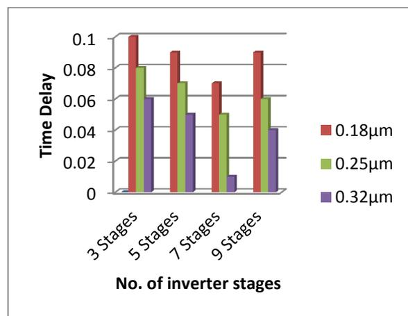
Fig. 4: Comparison chart for delay calculation for various stages in Ring Oscillator
