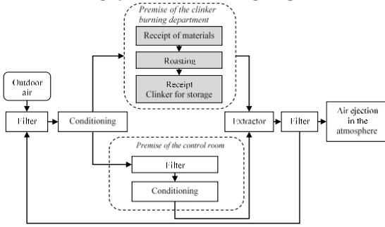
Fig.1. Block diagram of the heating, ventilating, and air conditioning system in the firing department
