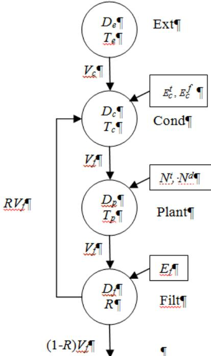
Fig. 2. The neighborhood structure of the ventilation-filtration system of a production workshop
