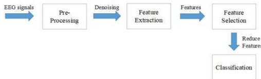
Fig. 2: Modules for the analysis of EEG Signals
