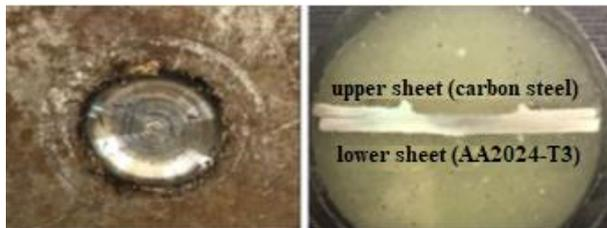
Fig. 9: Macrostructure Photographs of Cross-Section of Dissimilar FSSW Joints.
