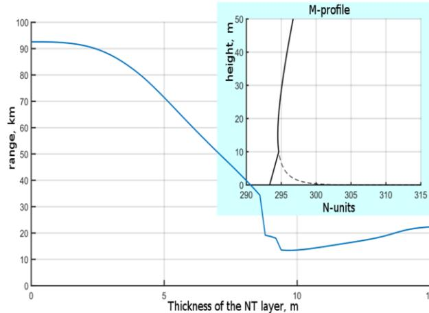
Fig. 5: Perturbing the profile of the evaporation-surface duct (see the inset at the top right of figure) and addition of the target detection ranges of the radar on the height of the section of the normal troposphere  $h_n$
