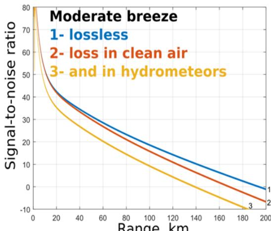
Fig. 3: Signal-to-noise ratio in evaporation duct in the moderate breeze.
