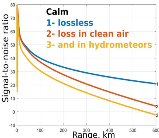
Fig. 2: Signal-to-noise ratio in evaporation duct in the calm.
