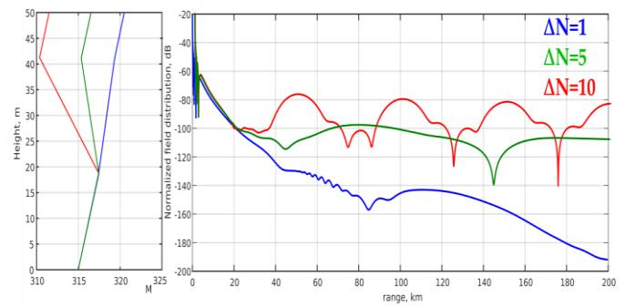
Fig. 6: The influence of the refractive index on radio propagation.
