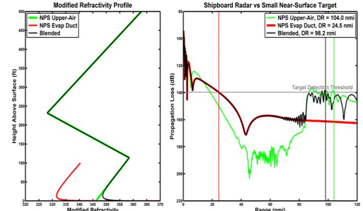
Fig. 8: Propagation loss calculated by P. Frederickson
