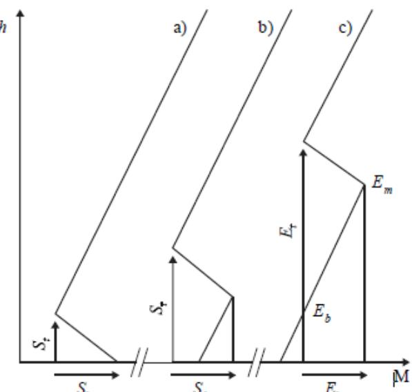
**Fig. 1:** Definition of parameters describing a) surface, b) elevated surface and c) elevated ducts
