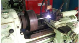
Fig. 1 Experimental setup used for plasma assisted turning
