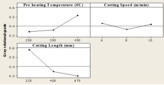
Fig. 4 Effect of turning control variable levels on multi performance
