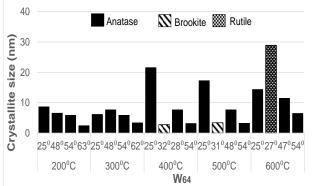
Fig. 6: Crystallite Sizes for TiO\_2 Coating Deposited with  $W_{64}$  Formulation Heated in the Range of  $200^{0}\text{C}\text{-}600^{0}\text{C}.$
