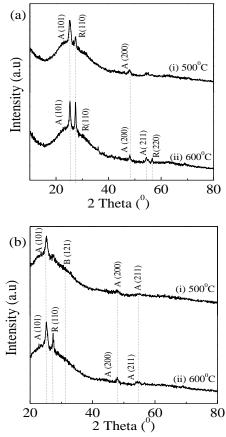
Fig. 1: XRD Patterns of the TiO<sub>2</sub> Thin Film Deposited with (A)  $W_{32}$  and (B)  $W_{64}$  Formulations Heated at (i) 500°C and (ii) 600°C (A=Anatase, R=Rutile and B=Brookite).
