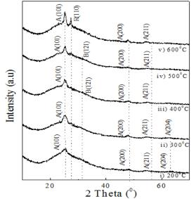
**Fig. 4:** XRD Patterns of the  $TiO_2$  Thin Films Deposited with  $W_{64}$  Formulation Heated in the Range of 200°C - 600°C (A = Anatase, B = Brookite, R = Rutile).
