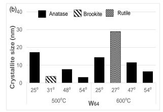
Fig. 3: Crystallite Size of the TiO<sub>2</sub> Deposited with (A)  $W_{32}$  and  $W_{64}$  Formulation Heated at 500<sup>0</sup>C and 600<sup>0</sup>C.
