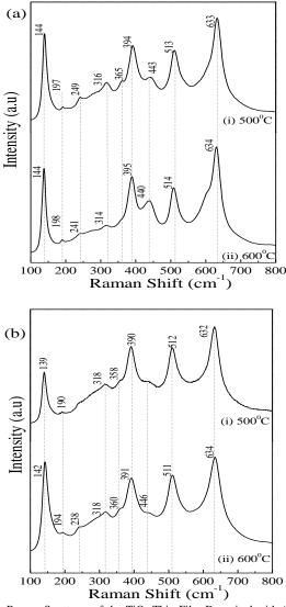
Fig. 2: Raman Spectrum of the TiO<sub>2</sub> Thin Film Deposited with (A)  $W_{32}$  and (B)  $W_{64}$  Formulations Heated at (i) 500°C and (ii) 600°C (A=Anatase, R=Rutile and B=Brookite).
