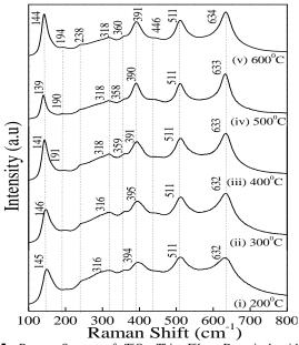
Fig. 5: Raman Spectra of TiO<sub>2</sub> Thin Films Deposited with  $W_{64}$  Formulation Heated in the Range of 200<sup>o</sup>C-600<sup>o</sup>C.
