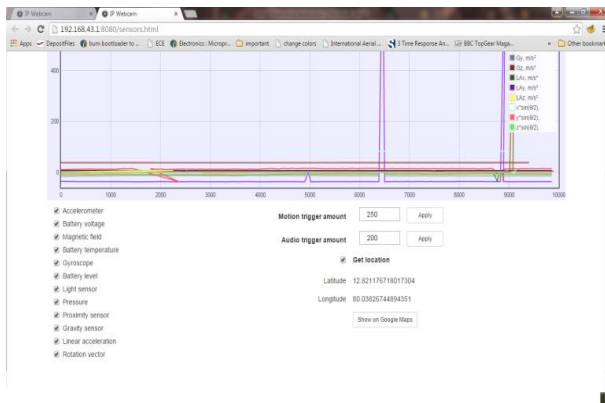
Fig. 32: GUI representing the entire Sensor Graphs Along with Latitude and Longitude Values
