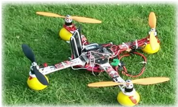
Fig. 2: The Plus Chassis of the Structure.
