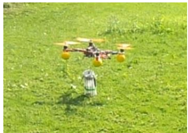
Fig. 35: Quadcopter is Taking Off with a Satellite Payload.
