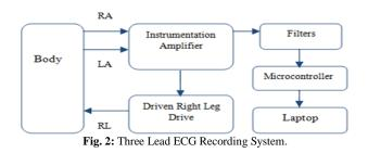
The ECG recording system used in this work is light weight and easily portable device. This device can be placed at the patient side for capturing the real time ECG signals .For transmitting the signals to nearby PHC this recording system can be interfaced with wireless module. Among the different wireless technologies available Zigbee technology is used here to transmit ECG signals to PHC.
