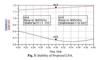
Therefore, the above obtained values of K > 1, B = +ve,  $|\Delta| < 1$  and  $\mu > 1$  proves that the device is unconditionally stable.
