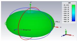
Fig. 11: Gain in ISM Band- 2.43 GHz.
