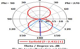
Fig. 16: Angular Plot for Gain at 2.43 GHz.
