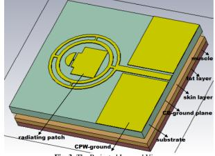
Fig. 3: The Projected Layered View.
