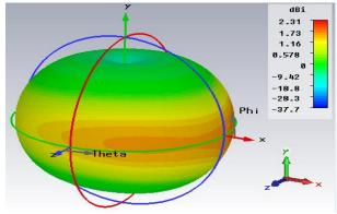
Fig. 12: Directive Gain in ISM Band - 2.43 GHz.
