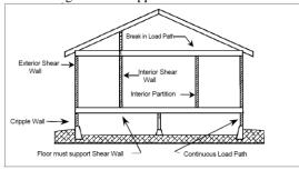
Fig.4: Horizontal alignment of cripple walls
