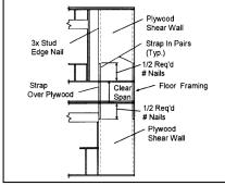
Fig.5: Vertical offset of shear walls
