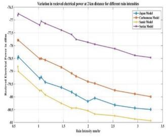
Fig. 7: Variation in received electrical power for single channel system
