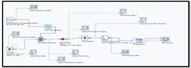
Fig. 1: Single Channel FSO communication system
