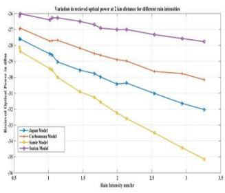
Fig. 5: Variation in received optical power for a single channel system
