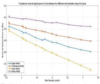
Fig. 6: Variation in received optical power for multiple channel system
