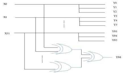
Fig. 3: architecture of CAC encoder (32, 97)
