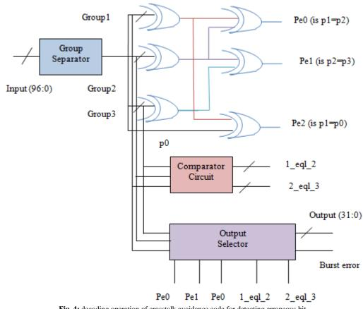
Fig. 4: decoding operation of crosstalk avoidance code for detecting erroneous bit
