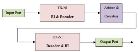
Fig. 2: Advanced NoC switch architecture with low power code with CAC codec components
