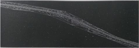
Fig. 5: Triangulation of all points within boundary
