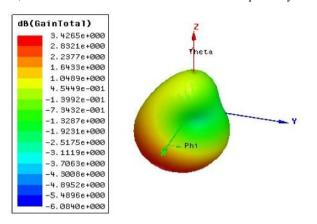
Fig. 15: Gain of antenna at frequency 3.3GHz
