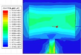
Fig. 4:Current Distribution on patch at f:5.2GHz.
