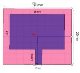
Fig.1: Front View of Antenna Without slots
