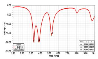
Fig. 11: Simulation of return loss of antenna with DGS
