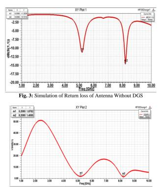
Since 5.2GHz is hold for WLAN application our aim is to keep grip of 5.2GHz and acquire other useful frequencies. This is completed according to the current distribution where slots are sliced in ground plane at less radiating part of 5.2GHz.
