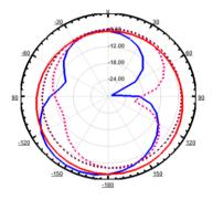
Fig.12: Radiation pattern at frequency 3.3GHz.
