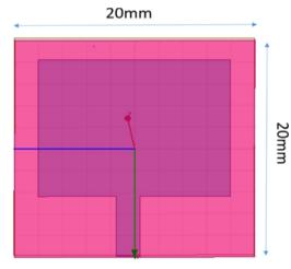
Fig. 2: Back View of the Antenna without slots
