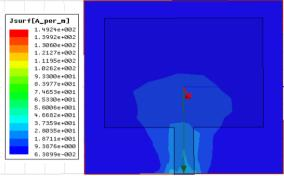
Fig. 5: Current Distribution on patch at f:3.3 GHz
