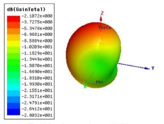
Fig. 16: Gain of antenna at frequency 3.85GHz
