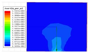
Fig. 6: Current Distribution on ground plane at f:3.3 GHz.
