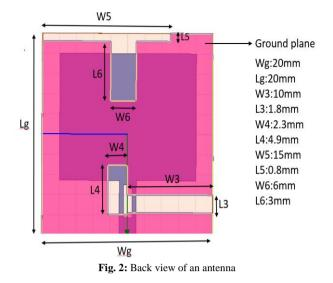
The L and T shape slots have been made in the ground plane to achieve multiple frequencies as depicted in the figure 2. All slot dimensions are balanced according to the length and width.
