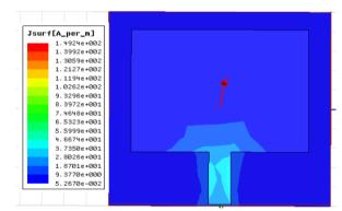
Fig. 8: Current distribution on patch at f:3.8GHz.
