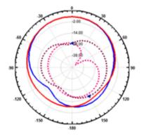
Fig.14: Radiation Pattern at frequency 5.25GHz
