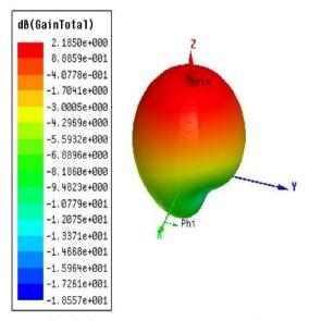
Fig. 17: Gain of antenna at frequency 5.25GHz
