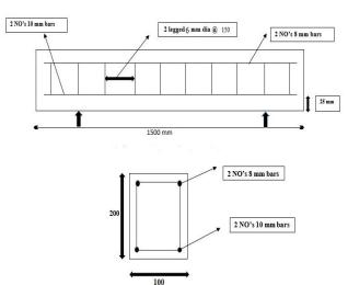
Fig. 1: Reinforcement details of beam
