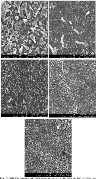
Fig. 2: FESEM images of ZnO nanostructures at b) 200, c) 300, c) 400 and d) 500  $^{\circ}$ C post-annealing temperature using TCVD while a) as-deposited sample
