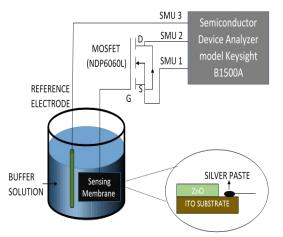
Fig. 1: EGFET pH sensing setup using semiconductor device analyzer (Keysight, B1500A)
