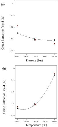
**Fig. 2:** (a) Effect plot of pressure (A) on crude extraction yield. (b) Effect plot of temperature (B) on crude extraction yield.
