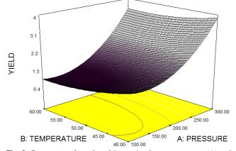
**Fig. 3:** Response surface plot of interaction between pressure (A) and temperature (B) on crude extraction yield.
