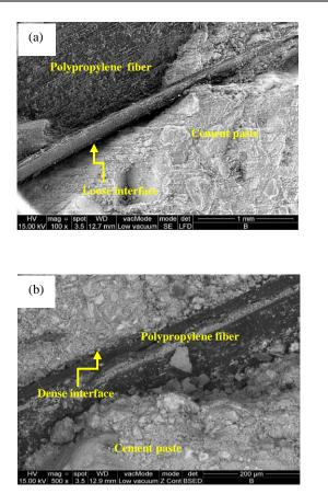
**Fig. 5:** Interface between the polypropylene fiber and cement paste at (a) 28 days and (b) 300 days
