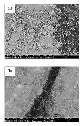
Fig. 2: Roles of (a) polyolefin and (b) polypropylene fibers in resisting crack propagation
