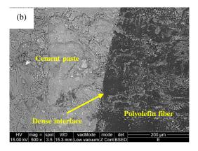
Fig. 4: Interface between the polyolefin fiber and cement paste at (a) 28 days and (b) 300 days
