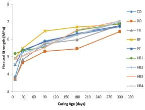
Fig. 3: Flexural strength versus curing age of tested specimens
