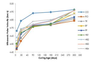
Fig. 6: Ultrasonic pulse velocity versus curing age of tested specimens
